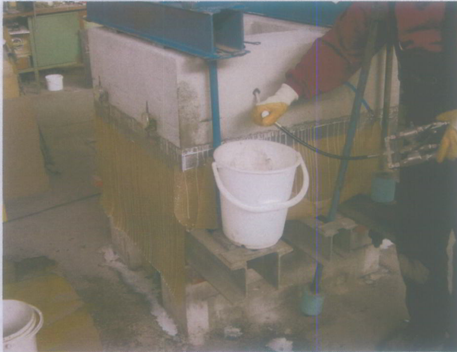
Fig. 7: 2nd sealing test specimen when injecting with DRYflex 2 / DRYflex plus
